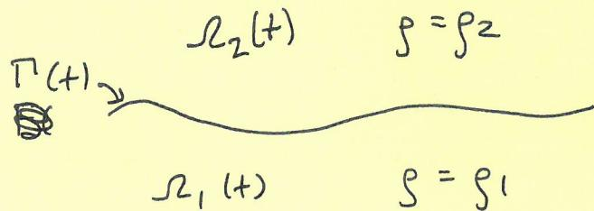
When the Euler equations are our basic model in each fluid region, this is sometimes called a "water wave problem", because it is a common model for the configuration
