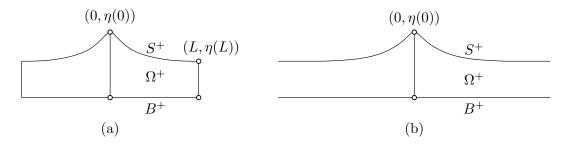
Figure 1: (a) The half-period  $\Omega^+$  of the fluid domain, together with the portions  $S^+$  and  $B^+$  of its boundary on the free surface and bed. (b) Analogous definitions for a solitary wave.
